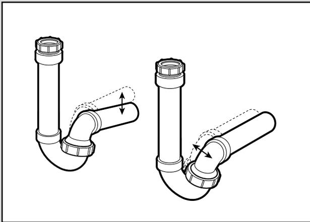
The ball joint union connection allows the P Trap Elbow to swivel up to 10° from vertical, in any direction, except directly backwards.
