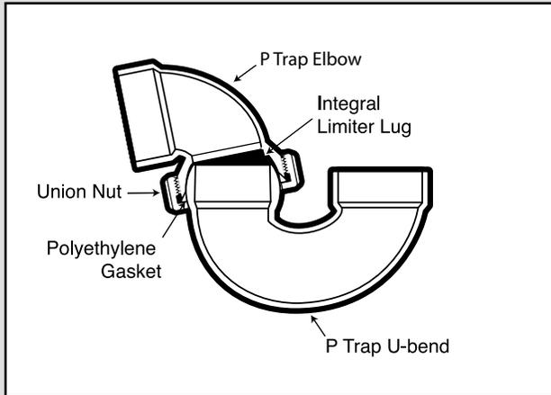
An integral limiter lug prevents the P Trap Elbow from pitching backwards providing the correct outlet slope for drainage. The polyethylene gasket ensures a leak proof connection in almost any installation situation.
